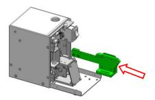
2. Install the feeding structure, and then fasten screw.
