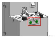
2. Make sure to cover half of the hole, and then fasten the screw of step 1.
