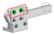
2. Adjust the height of holding plate by tooling plate, and fasten the screw of step 1.
