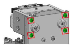
2. Adjust the groove of circled plate to the middle of rail, and then fasten the screws of step 1.
