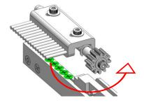
3. When fix the brush position, keep suitable space for the Front Plate and Fixing Plate.
