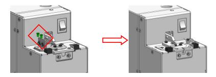
2. Remove the fixing screws (8pcs) of front housing, and take off the front housing.
