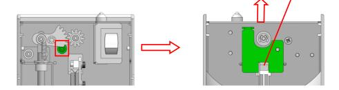
5. Remove the fixing screws of rail assembly
