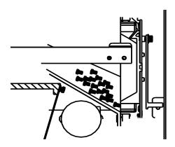
All objects other than applied screw are deemed as foreign material which should be removed first; or it will affect the performance of this machine.
