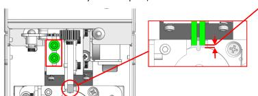
4. Set the lock gate, keep 0.2~0.5mm open space between gate to rail assembly.
