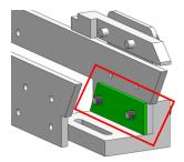
4. Insert the tooling plate in the rear end of rail according to Table b, fasten the screw of step 1.
