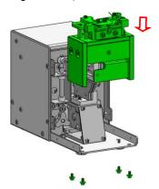
3. Loosen the fixing screw of rail assembly, keep  $0.2 \sim 0.5$ mm open space between the front end of rail assembly to circled plate, and then fasten screw.
