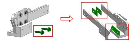
3. According to Table b, insert the suitable tooling plate into the rail groove for the width required and tighten the screw of step 2.
