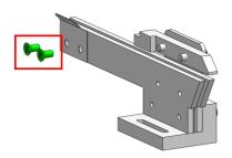
2. Remove the fixing screw on the front end of side of rail assembly, take off the tooling plate.
