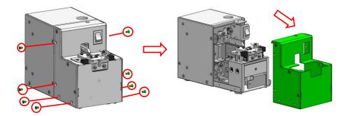
3. Dismantle the fixing screws\*4 of feeding structure, and take it off.
