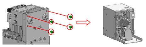
Facing the machine, loosen the screw of lock gate, open the lock gate upward and fasten screw.
