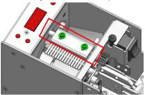
2. Place 5~8 screws into the rail groove close to the holding plate rear end, loosen 2 screws on the side of the brush bracket, swing the brush down and adjust the height, the brush just touch the screw heads slightly, and tighten the screws after adjustment.
