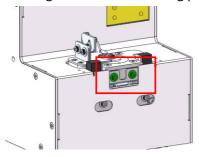
2. Make sure to cover half of the hole, and then fasten the screw of step 1.
