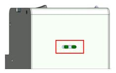
2. Adjust V Chase to face to the center of the rail. Distance between Chase and rail should be 0.8~1.0mm
