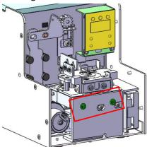
4. Adjust from part by up and down to make disc and rail flush, and then fasten loosen screw in step 3
