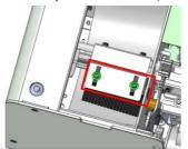
2. Place 5~8 screws into the rail groove close to the holding plate rear end and loosen 2 screws on the side of the brush bracket. Swing the brush and adjust the height until the brush just touch the screw heads slightly, and tighten the screws after adjustment.
