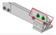
2. Use accessory tooling plate adjust height of force-down plate and then fasten screw in step 1
