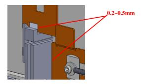
4. Loosen the fixing screw of rail assembly. Keep 0.2~0.5mm open space between the front end of rail assembly and circled plate. Then fasten the screws.
