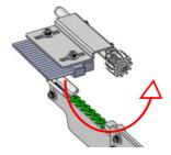
3. When fix the brush position, keep suitable space form the Front Plate and Fixing Plate.
