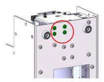
2. Align disc gap with central of rail by adjust front of distribution mechanism by left and right, Fasten the loosen screw in step 1
