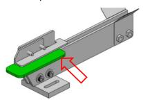
3. Put some screws into the groove and slide it up, to check whether the movement is smooth
