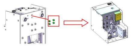
4. Facing the machine, use Hex wrench to loose the screw clockwise to open the lock gate upward.
