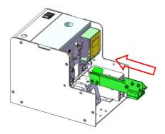
2. Install the feeding structure. Then fasten the screws.
