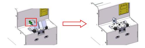
2. Remove the fixing screws (6pcs) of front housing, and take off the front housing.
