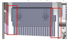
4. Brush bracket and driving rod must be parallel and fix to the center.
