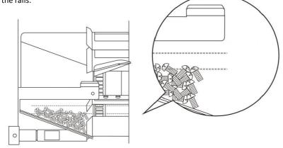
Can contain screws between 200~220cc. All objects other than applied screw are deemed as foreign material which should be removed first; or it will affect the performance of this machi
