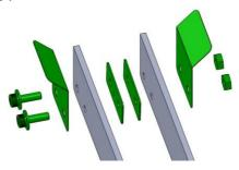
3. According to Table b, insert the suitable tooling plate into the front and rear end of the rail. Then adjust the width for left and right rail. Tighten the screw of step 1 and 2.
