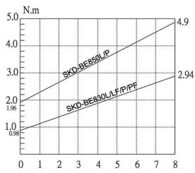
However, the clamping torque of screw itself is different form type, size, material of the screw and the material of its mating part. Use it as standard to obtain an appropriate clamping torque.
